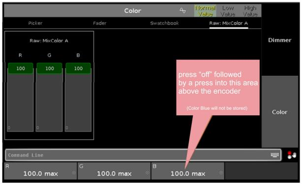
To switch a Color off, first press the "Off" button, followed by typing into the grey field above the encoder.
